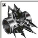
**LB205** - 22.2mm. Chainstays 60x64x7° angles. Slots and guides in bottom.
