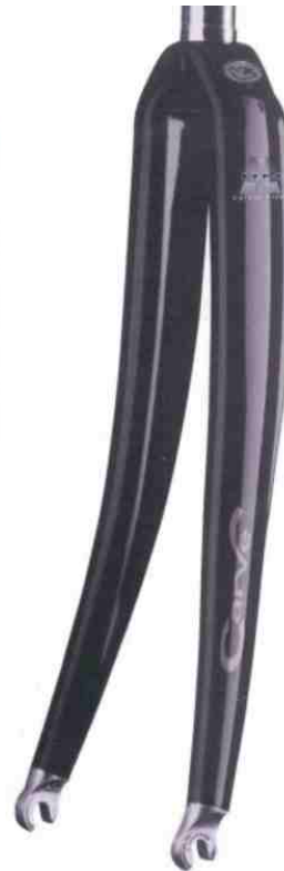
Carve 2004 - 28.6mm Integrated. 45mm offset. 300mm Carbon Steerer. Monocoque Single Piece Profiled Design. 420g Average
